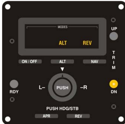
Fig. 2-24. AP Display, REV and ALT HOLD Modes Engaged, TRIM DN Required (System Fifty)
