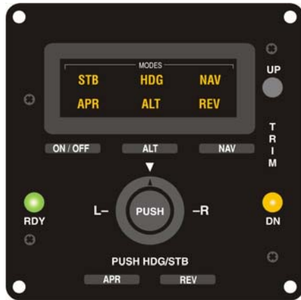
Fig. 2-11. AP Display, TRIM UP Lamp Extinguished (System Fifty)
