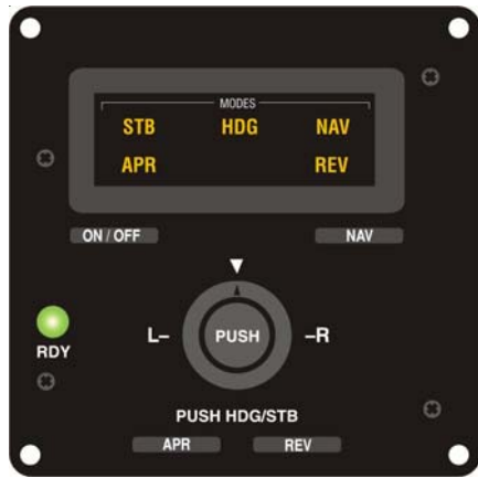
Fig. 2-1. AP Display, STB, HDG, NAV, APR, REV Annunciations Appear, RDY Lamp Illuminated (System Forty)
